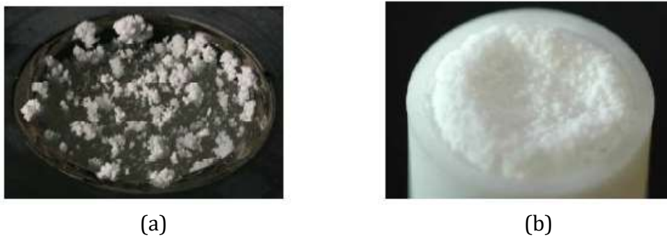
Figure 4- 8 : (a) Efflorescence chou-fleur. (b) Efflorescence croute [27].
